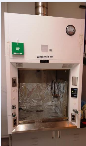
Figure 1: Dedicated Fumehood (Wetbench #9) for Nanoparticle Sample Preparation
