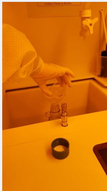
5. Put the cap back on the waste container. Make sure you do not overtighten the caps.
