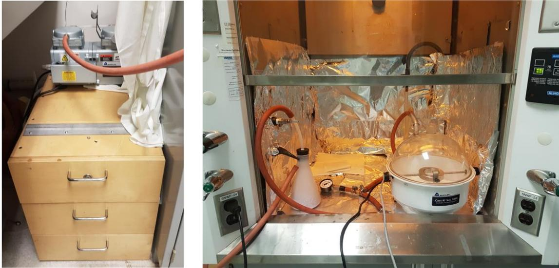
Figure 2: Embedding system set-up within the fume-hood
