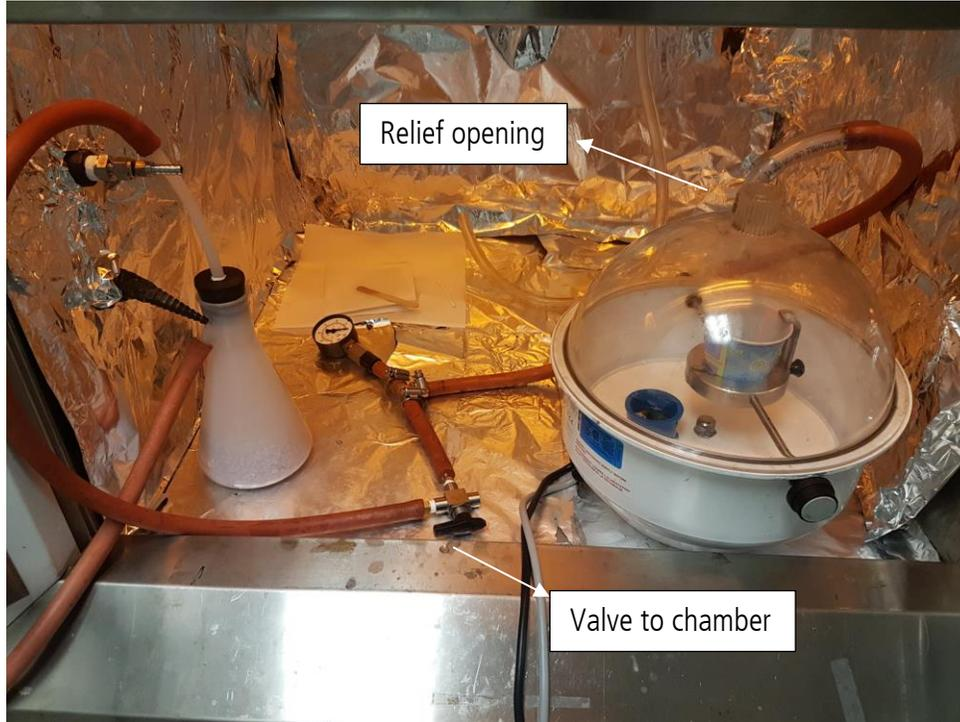
Figure 4: Embedding system set-up within the fume-hood with mold
