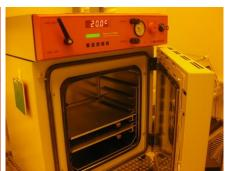
• Insert the sample, close the oven door, and open the vacuum valve.
