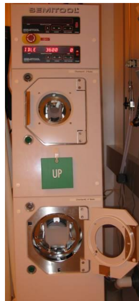
Figure 7: Wafer cassette in SRD.
