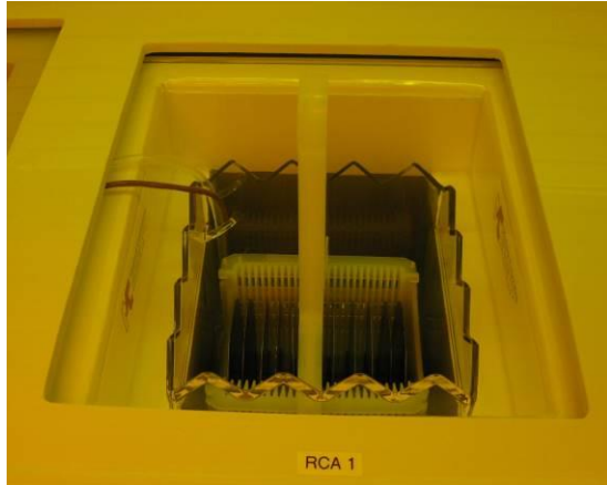
Figure 4: Wafer cassette in RCA-1 tank.
