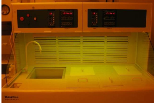
Figure 1: Overall view of RCA wet bench.
