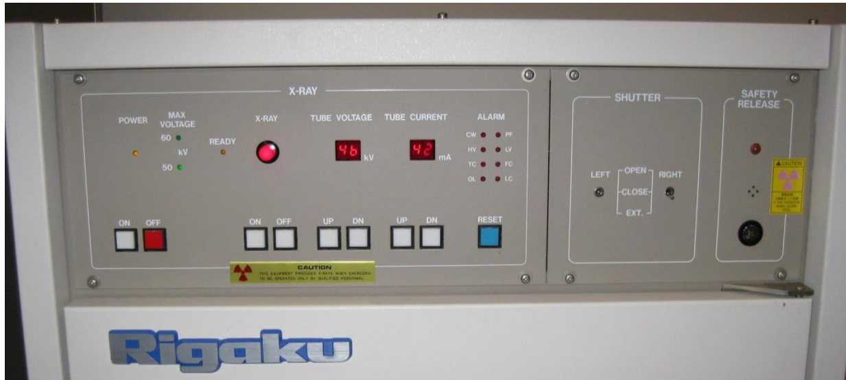
Figure 1: Top panel of the XRD1 electronics cabinet. Voltage and current are at full power (46 kV, 42 mA).
